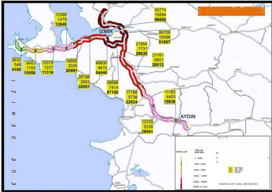
Figure 51. Highways 2nd Zone 2014 Highways Traffic Volume Map
